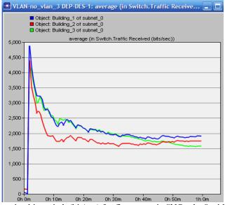
Figure 18: Traffic received in switch (bit/sec) for first scenario "NO\_vlan" with three departments.
